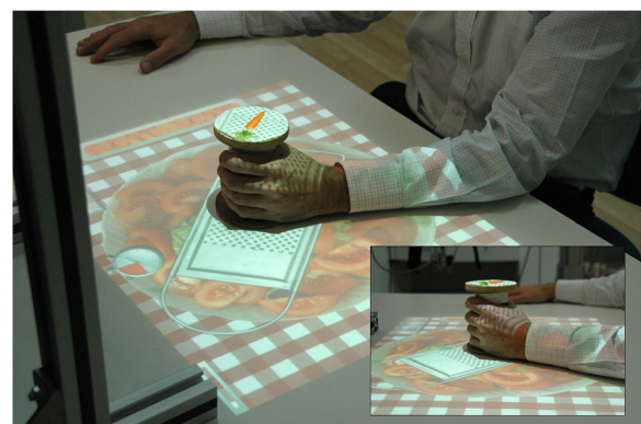
Fig. 2 Participant training with the system. A participant interacts with the system using a tangible object. Participant must grate a carrot, represented on the top surface of the item, on a salad. The task is achieved through repeated flexion-extension of the wrist, while maintaining the forearm on the table and the elbow still
