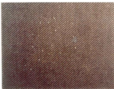
Figure A.1 – Photographic standard – friction medium I: Pilling grade 4–5
