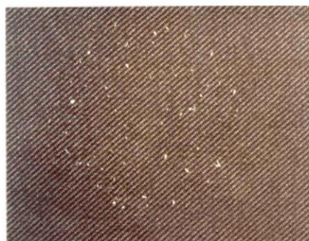
Figure A.2 – Photographic standard – friction medium I: Pilling grade 3–4
