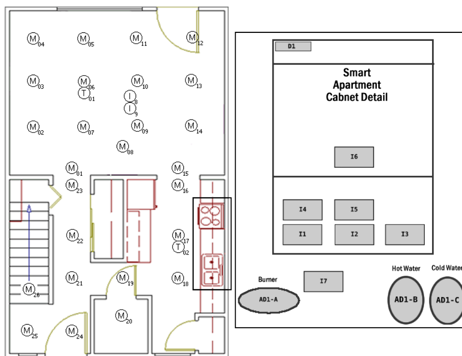
Figure 3.2: Sensor distribution for the testbed in OA and OA-E [23]
