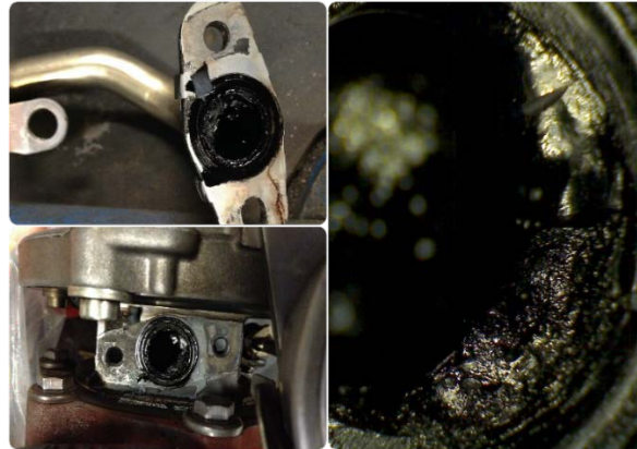
Figure 10. Oil coke deposits in a turbocharger tested at 2750 rpm- full load and oil type A with 7% of soot.
