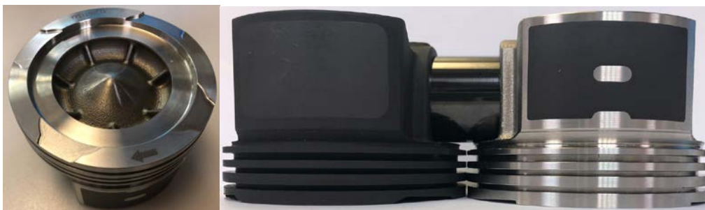
Fig. 3. Prototype steel piston left and side view (comparison with forged steel piston is provided, to show same compression height and top land).
