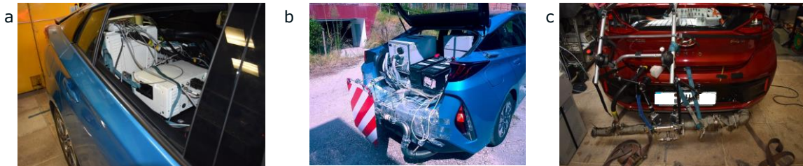
Fig. 5. Installation of PEMS on the vehicles used for the experimental campaign
