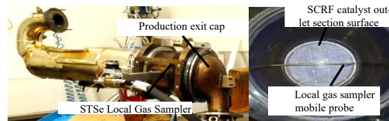
Fig.2. ATS installed in STSe HFB equipped with STSe Local Gas Sampler
