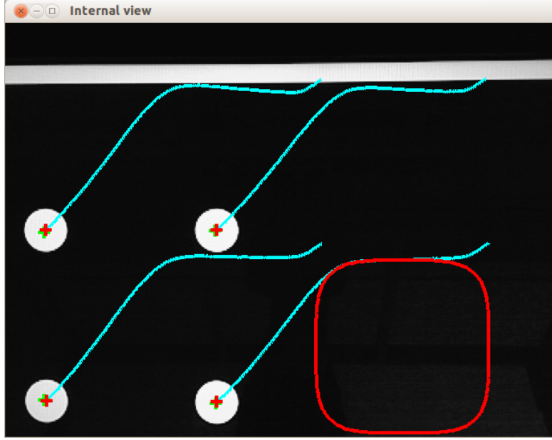
Fig. 18. Image features trajectories for the IBVS experiment with no errors in the gradient vector. Snapshot in the desired pose.
