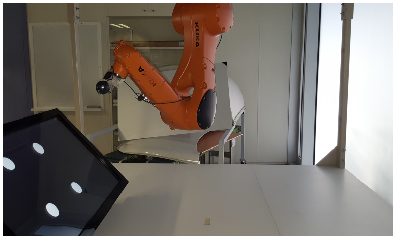
Fig. 13. Experimental setup: 6R serial industrial manipulator in ceiling position with the camera rigidly attached to the robot end-effector (eye-in-hand) and a screen to display the object markers.
