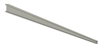
Fig. 4. Representation of the I-shaped spar of Drone Mermoz's wing
