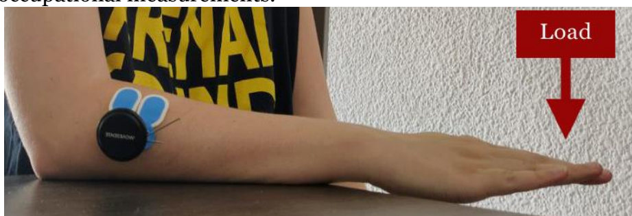
Fig. 15. Placement of the arm and the wrist during the second experiment and where the load was placed.
