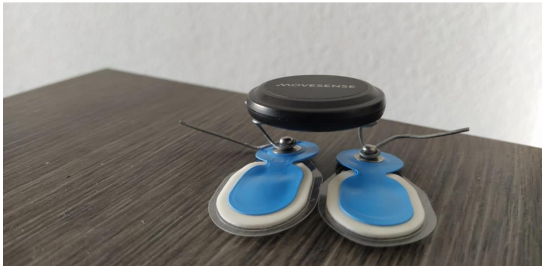
Fig. 13. The electrodes and the sensor with the developed wire structure.
