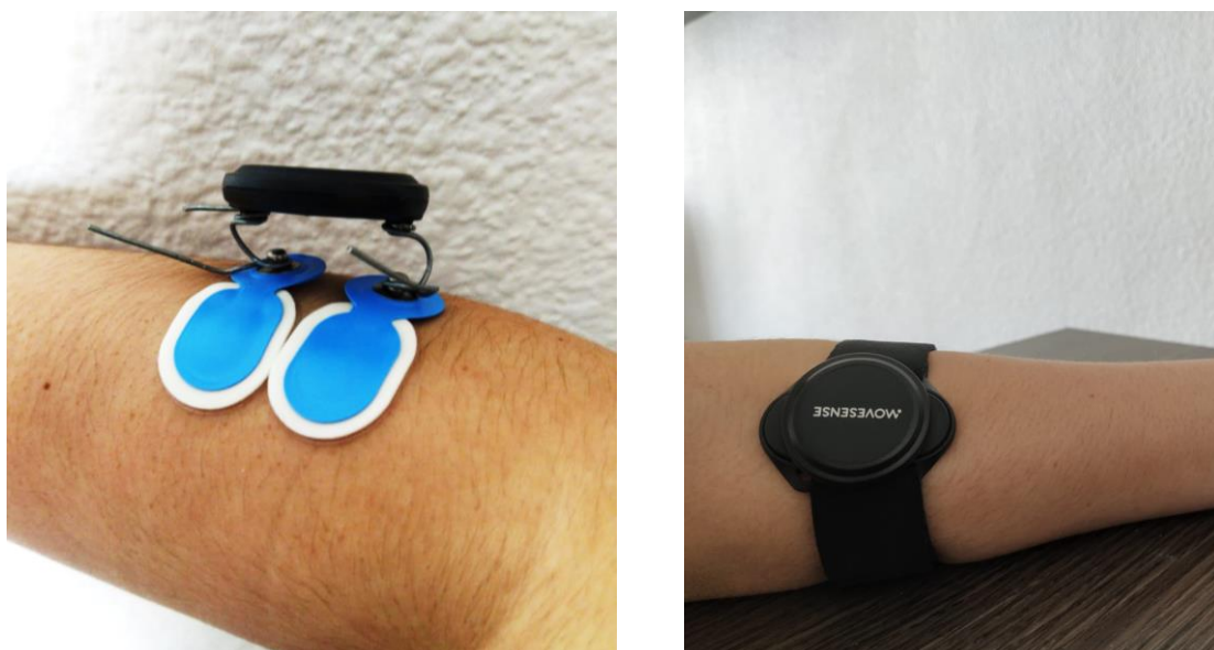
Fig. 14. Placement of the sensor with the electrodes (left) and with the elastic band (right).
