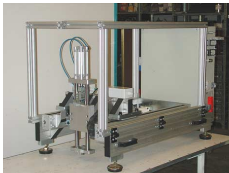
Fig. 2. DCOF device. The set has retractable wheels for being portable. When the device is on the test surface it rests on four rubber supports to reduce vibrations (device dimensions: base: 711 \times 980 mm; high: 813 mm; weight: 95 kg).
