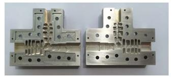
Fig. 11. Photograph of the unassembled prototype fabricated by computercontrolled milling in aluminum in clam-shell configuration.
