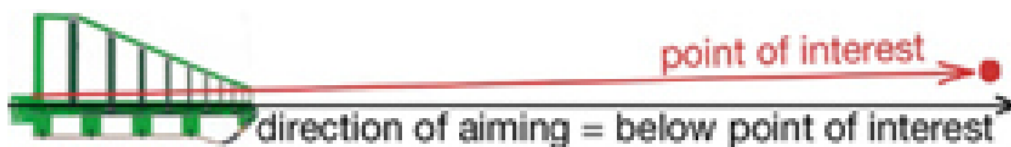
Figure 4.8: Scheme of the correct antenna pointing 10° over the point of interest
