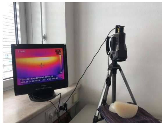
Figure 39: Side cut of agar phantom viewed through infrared camera
