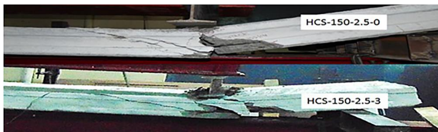
Figure 2-42: MOF of the SFRC hollow core slab [192]
