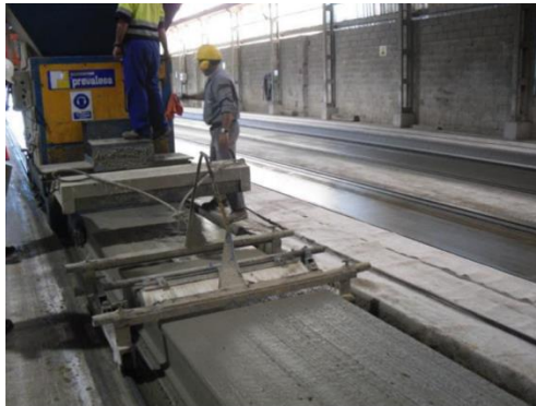
Figure 2-38: Extrusion process of HCS [185]
