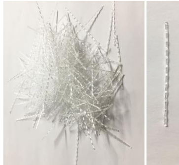
Figure 5-4: The employed crimped polypropylene fibres
