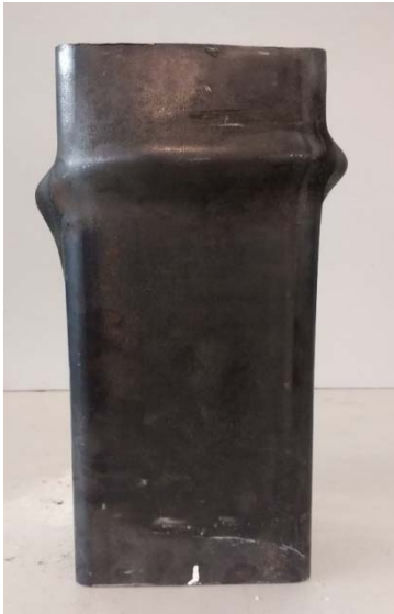
Fig. 4. Typical failure mode (S125x125x3_30)
