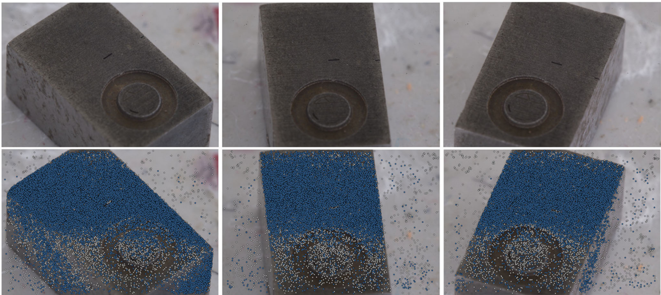
Fig. 4 Above, example of three pictures taken from different positions and below, tie points recognized on them
