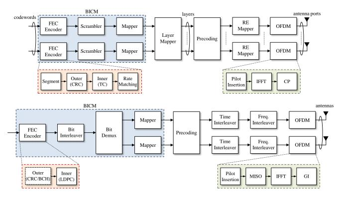
Fig. 1. LTE-Advanced Pro eMBMS (top) and ATSC 3.0 (bottom) physical layer transmitter block diagram.
