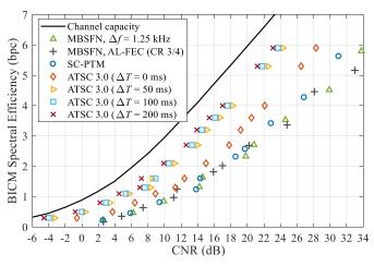
Fig. 7. BICM spectral efficiency vs. CNR in dB of LTE-Advanced Pro Rel-14 MBSFN, SC-PTM and ATSC 3.0. TU-6 mobile channel with 120 km/h at 700 MHz carrier frequency.
