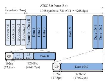
Fig. 2. Maximum number of data cells in the ATSC 3.0 frame.
