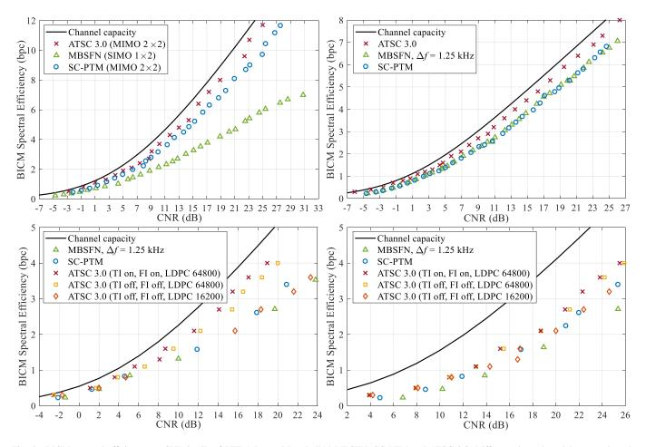
Fig. 5. BICM spectral efficiency vs. CNR in dB of LTE-Advanced Pro Rel'14 MBSFN, SC-PTM and ATSC 3.0. Different channel models are evaluated: i.i.d. Rayleigh MIMO channel (top left), DVB-F1 Rice (top right), NGH-PO (bottom left) and NGH-PI (bottom right).
