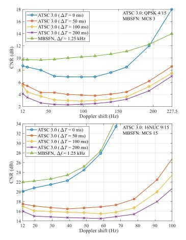
Fig. 8. CNR to achieve a BLER 0.1% against user speed, for SC-PTM, MBSFN and ATSC 3.0 in TU-6 mobile channel. MCS 3 vs. QPSK 4/15 (top) and MCS 15 vs. 16NUC 9/15 (bottom).
