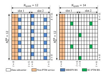
Fig. 3. MBSFN (left) and SC-PTM (right) frame configurations. Both employ a carrier spacing of 15 kHz.
