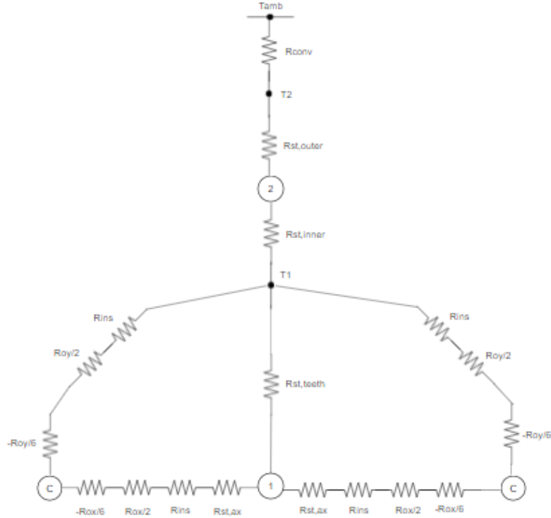
Figure 6.3: Equivalent thermal network for the simplified generator
