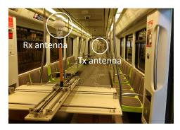
Fig. 1. Interior view of the convoy with the Tx and Rx antennas.
