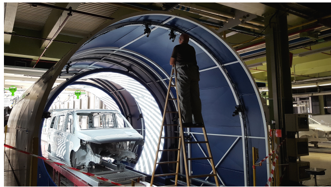
(c) Expert performing the camera 3D positioning task in the QEyeTunnel system.
