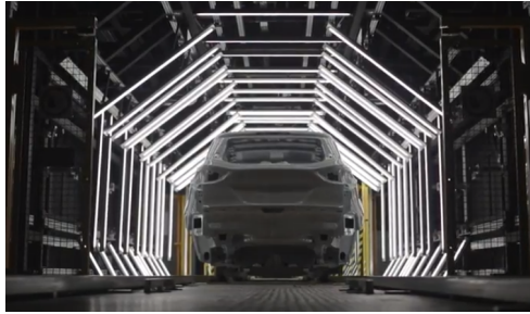
(a) AIS system developed in Ford factories https://www.youtube.com/watch?v=HroEU8XsaTU . (b) QEyeTunnel system developed in Mercedes factories https://www.youtube.com/watch?v=jN8vazudEXc .
