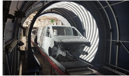
(a) AIS system developed in Ford factories https://www.youtube.com/watch?v=HroEU8XsaTU . (b) QEyeTunnel system developed in Mercedes factories https://www.youtube.com/watch?v=jN8vazudEXc .
