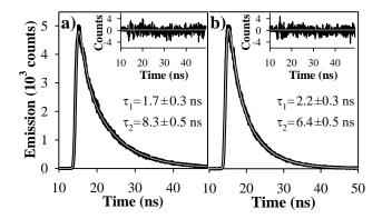
Figure 11. Emission decays recorded at 450 nm ( $\lambda_{exc}$  = 341 nm). Insets: residual analysis. a) DNA samples irradiated in the presence of Ptr under anaerobic conditions. [Ptr]<sub>0</sub> = 150  $\mu$ M, [DNA]<sub>0</sub> = 150  $\mu$ M bp, pH = 6.5±0.1. b) dT<sub>5</sub> samples irradiated 60 min in the presence of Ptr under anaerobic conditions. [Ptr]<sub>0</sub> = 150  $\mu$ M, [dT<sub>5</sub>]<sub>0</sub> = 50  $\mu$ M, pH = 5.5±0.1.
