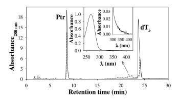
Figure 6. HPLC analysis of an air-equilibrated solution containing  $dT_5$  and Ptr before (solid line) and after 40 min (dashed line) of irradiation. Chromatograms obtained using the PDA detector at 280 nm. Insets: absorption spectra of the products and detail in the range 300-420 nm. [Ptr]<sub>0</sub> = 150  $\mu$ M, [ $dT_5$ ]<sub>0</sub> = 50  $\mu$ M, pH = 5.5±0.1.
