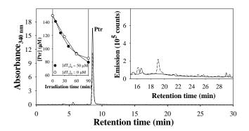
Figure 7. HPLC analysis of an air-equilibrated solution containing  $dT_5$  and Ptr before (solid line) and after 40 min (dashed line) of irradiation. Chromatograms obtained using the PDA detector at 340 nm. Left inset: evolution of the Ptr concentration as a function of irradiation time; right inset: chromatograms obtained using the fluorescence detector (excitation at 350 nm, emission at 450 nm);  $[Ptr]_0 = 150 \mu M$ ,  $[dT_5]_0 = 50 \mu M$ , pH = 5.5±0.1.
