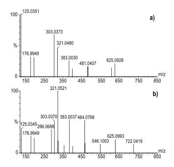
Figure 5. MS/MS spectra recorded in ESI<sup>-</sup> mode of a) the di-charged ion of dT<sub>5</sub> ([dT<sub>5</sub>-2H]<sup>2-</sup> and b) the di-charged ion of the product with  $t_r$  at 7.3 min ([dT<sub>5</sub>+Ptr-4H]<sup>2-</sup>). Analysis of a solution containing dT<sub>5</sub> and Ptr after 40 min of irradiation under anaerobic conditions.
