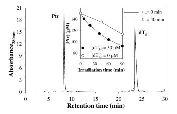
Figure 2. HPLC analysis of a solution containing  $dT_5$  and Ptr before (solid line) and after 40 min (dashed line) of irradiation under anaerobic conditions. Chromatograms obtained using the PDA detector at 280 nm. Inset: evolution of the Ptr concentration as a function of irradiation time. [Ptr]<sub>0</sub> = 150  $\mu$ M, (o) [ $dT_5$ ]<sub>0</sub> = 0  $\mu$ M, ( $\bullet$ ) [ $dT_5$ ]<sub>0</sub> = 50  $\mu$ M, pH = 5.5±0.1.
