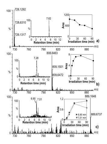
Figure 4. Mass spectrometry analysis of a solution containing  $dT_5$  and Ptr after 40 min of irradiation under anaerobic conditions. MS spectra (ESI mode) of the di-charged ions of: a)  $dT_5$ ; b) the product with  $t_r$  at 7.3 min; c) the product with  $t_r$  at 6.9 min. Insets: mass chromatograms for the specific ion mass of a)  $[dT_5-2H]^{2-}$ ; b)  $[dT_5+Ptr-4H]^{2-}$ ; c)  $[dT_5+2Ptr-6H]^{2-}$  and evolution of the area of the corresponding peaks as a function of irradiation time.
