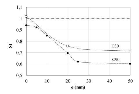
Fig. 7. Strength index (SI) vs eccentricity.
