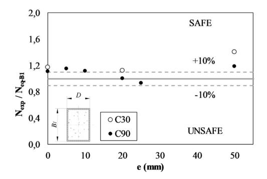
Fig. 16. Comparison between proposal B1 predictions and experimental ultimate loads.
