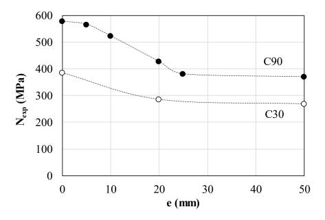
Fig. 5. Ultimate load vs eccentricity.
