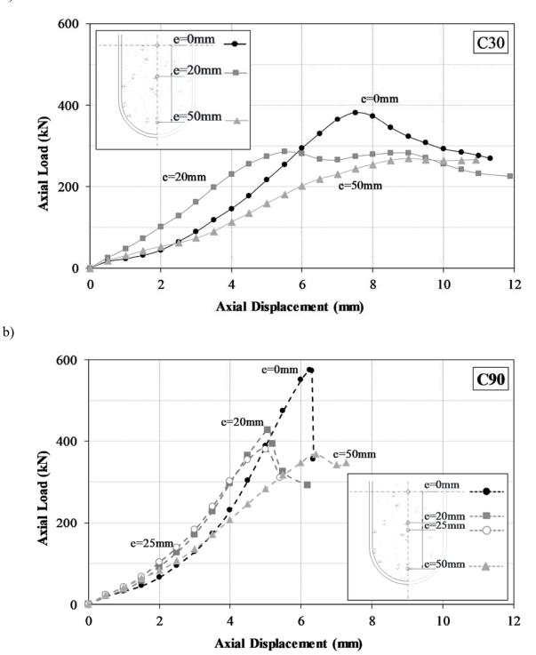
Fig. 6. Compression load versus shortening for: a) Series 1 C30; b) Series 2 C90.
