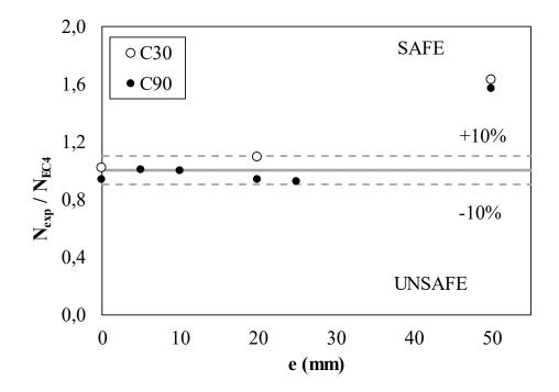
Fig. 12. Comparison between EC4 predictions and measured cross-sectional strengths.
