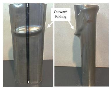
Fig. 4. Typical failure mode.
