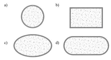
Fig. 1. Different cross-sectional shapes for CFST columns: a) Circular; b) Rectangular; c) Elliptical; d) Round-ended.
