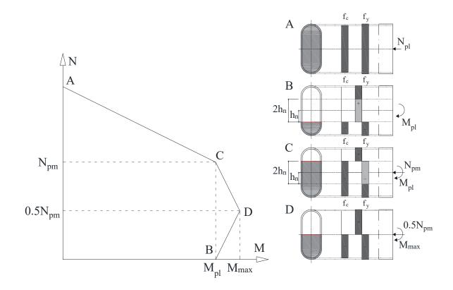
Fig. 10. M-N interaction curve determination according to EC4.
