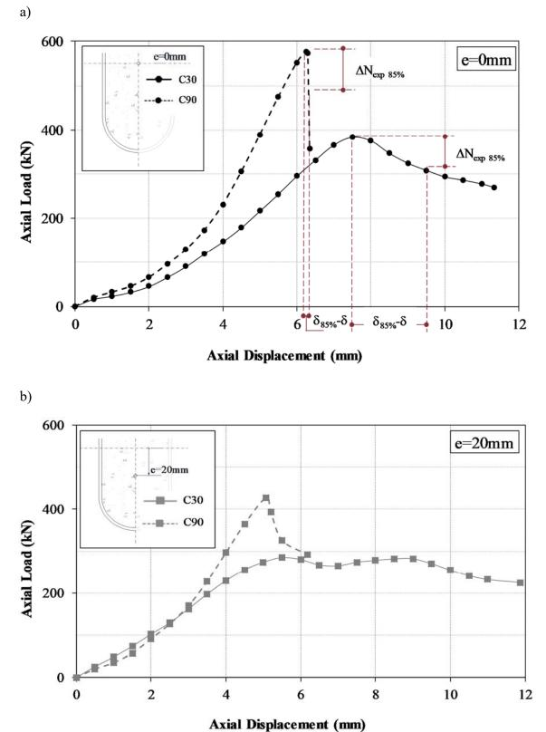
Fig. 9. Determination of ductility index from load-shortening curves: a) Columns RND 30 00 and RND 90 00; b) Columns RND 30 20 and RND 90 20.
