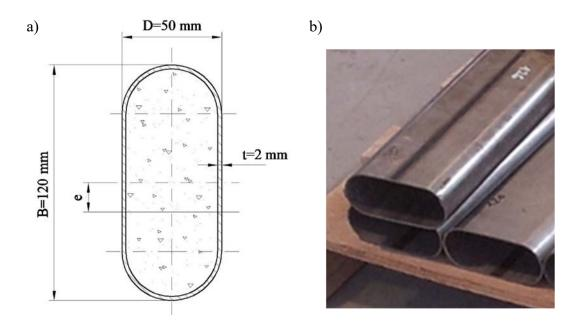
Fig. 2. Column cross-section: a) Dimensions; b) Round-ended hollow steel sections.
