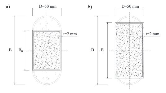
Fig. 13. Equivalent rectangular CFST cross-sections analysed.
