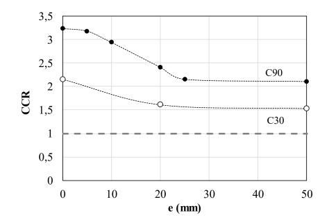
Fig. 8. Concrete contribution ratio (CCR) vs eccentricity.
