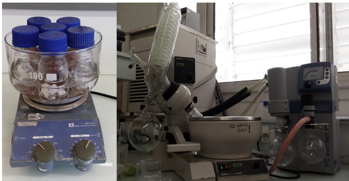
Figure 6-4 - Rotavapor extraction system and vacuum unit used to foulants extraction, used in the IEM.
