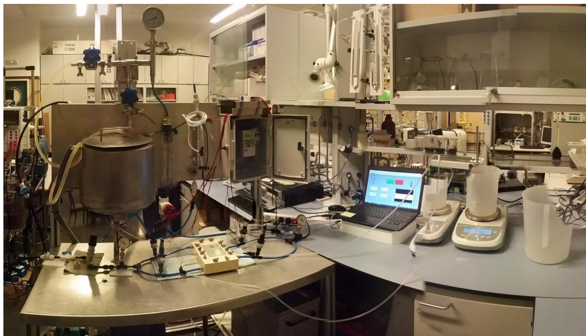
Figure 3-6 - Photographs of the experimental system. UF pilot plant with flat-sheet membrane module (Rhône-Poulenc, France).
