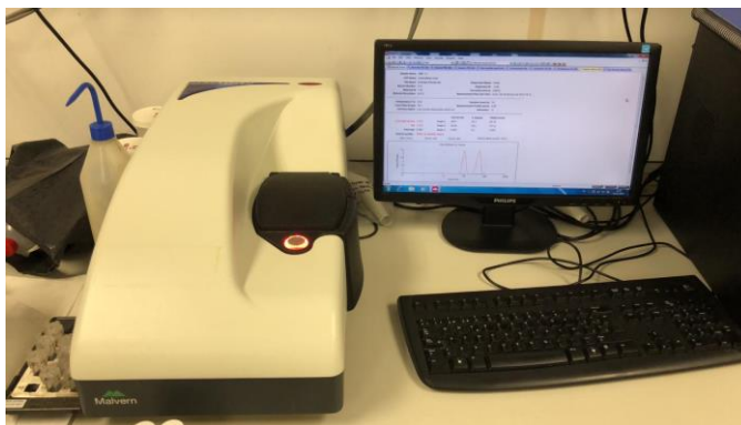
Figure 3-3 - Photograph of the setup for Zetasizer Nano ZS instrument (Malvern Instruments) used in the ISIRYM.
