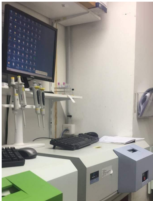
Figure 6-5 - Photograph of Perkin-Elmer, LS-55 fluorescence spectrometer (Perkin-Elmer, USA), used in the IEM.
