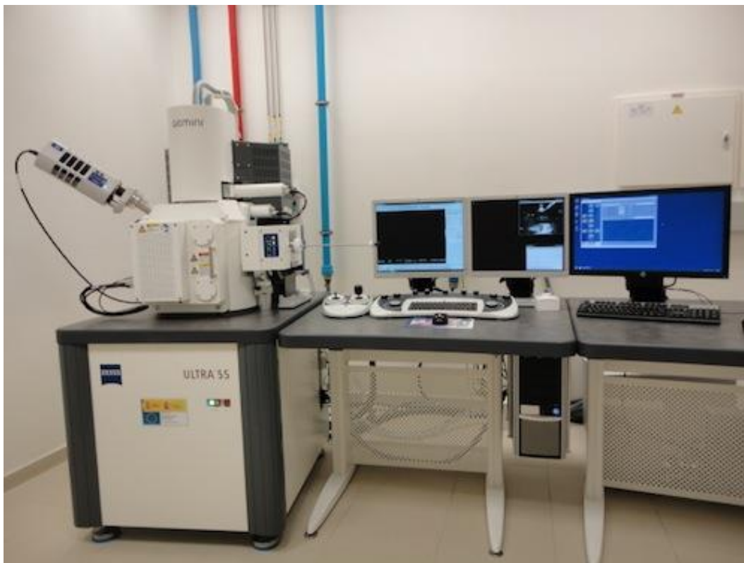
Figure 6-2 - Field Emission Scanning Electron Microscope (FESEM) (ZEISS ULTRA 55 model. Oxford Instruments, UK) used in the ISIRYM.
