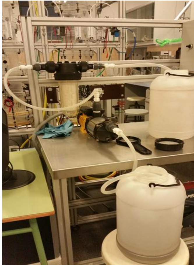
Figure 3-5 - Schematic image of the setup with a conventional filtration used for pre-treatment before the cross-flow UF.
