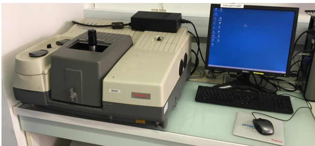
Figure 6-3 - FT-IR spectrometer with universal ATR Sampling Attachment (Thermo Electron Corporation, USA) used in the IEM.
