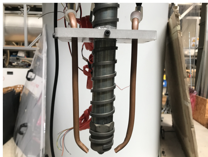
Figure 3.7 : Closer shot at the bottom of the extruder
