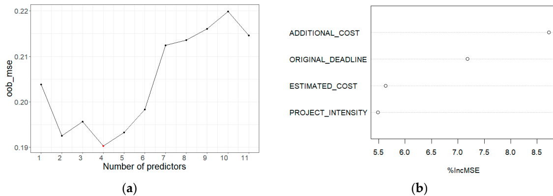
Figure 6. Optimal number of predictors (a) and significant variables (b) for time deviation.
