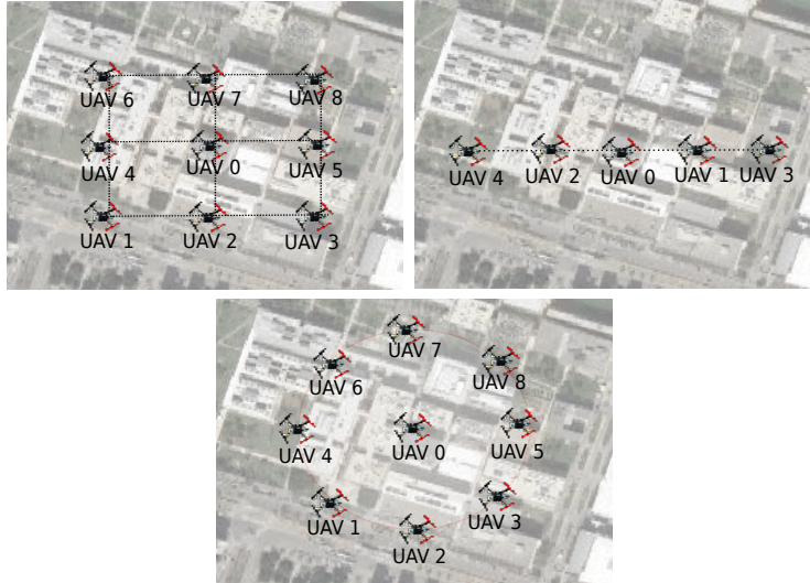
Figure 6: Different swarm layouts tested: i) matrix with 9 UAVs, ii) linear with 5 UAVs, and iii) circular with 9 UAVs.
