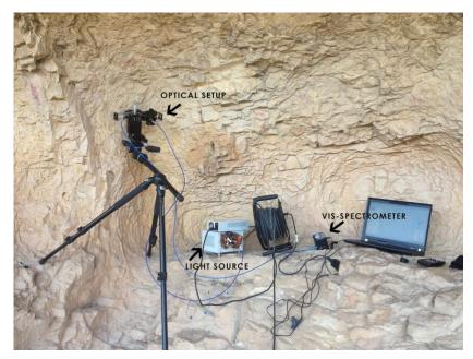
Figure 1. MFT setup used for the light stability evaluation of rock art paintings.
