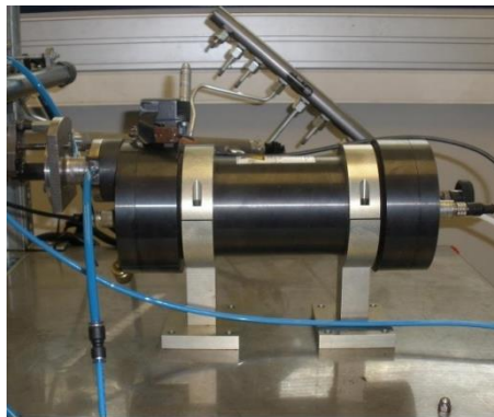
Figure 2: EVI injection rate meter
