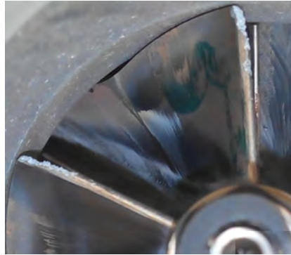
Figure 9: Noticeable erosion detected after 50 hours of testing.
