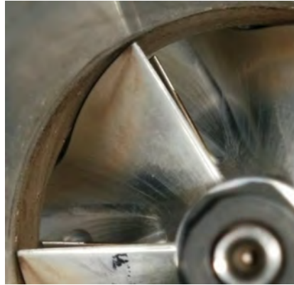
Figure 7: No erosion detected after 50 hours of testing.
