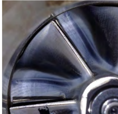
Figure 8: Slight erosion detected after 50 hours of testing.
