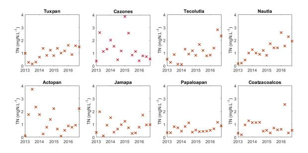
Figure 5.5: Total nitrogen concentrations in all monitoring sites, between 2013 and 2016 with four values per year
