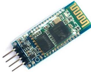
Figura 13. Módulo bluetooth HC-06 [21]
