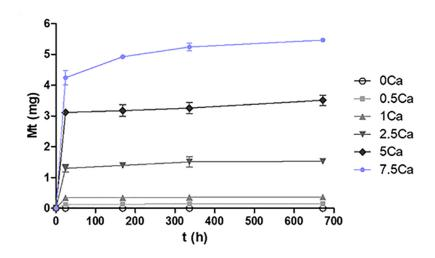
Fig. 2. Kinetic liberation of  $Ca^{2+}$  from the coatings. Mt represents the total amount of  $Ca^{2+}$  release from the sol-gel network during time.
