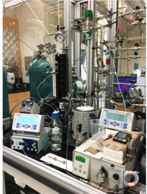
Figure 14. Process flow diagram and experimental setup of the packed bed reactor process for continuous-flow \beta -lactone carbonylation.
