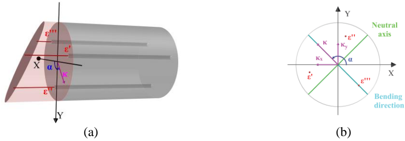
101 Fig. 1. (a) 3D Strain distribution for a generic sensor where the strain is sensed at 3 points, by way of example; (b) 102 Cross section. 103 104
