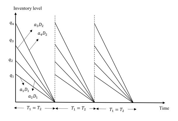
Fig 3. Inventory model diagram for situation 3.  $(T_1 = T_2)$
