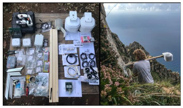
Fig. S1.5. Left: material used to build some of the installed meteorological stations. Right: installation of a meteorological station.
