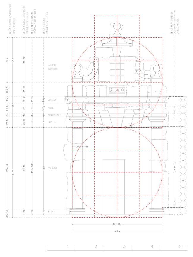
Fig.6 Main front, of the Tuscan Vignolesque order. Its dimensions are delimited in the Valencian metric pattern and in the module that corresponds to the semi-diameter of the column –pilastra-, according to Vignola and according to Fray Lorenzo de San Nicolás (Authors 2013).
