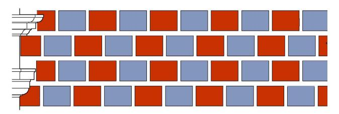
Fig. 17. View of the beginning of the stakeout of the fake ashlars, from the south flank to the left of the facing (Authors 2013).
