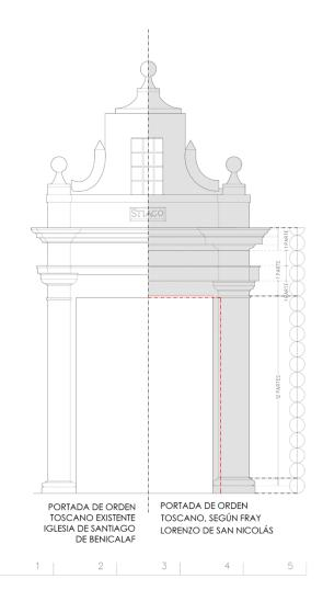
Fig. 9. Comparative drawing between the real cover –left– and the one that, observing the proportions of Fray Lorenzo de san Nicolás, would have been –right–. The similarity in the height of the column shaft and in the coincidence of lines in the upper part of the architrave and cornice stands out. In red strokes, on the right cover, the current doorway is hinted at. (Authors 2013).
