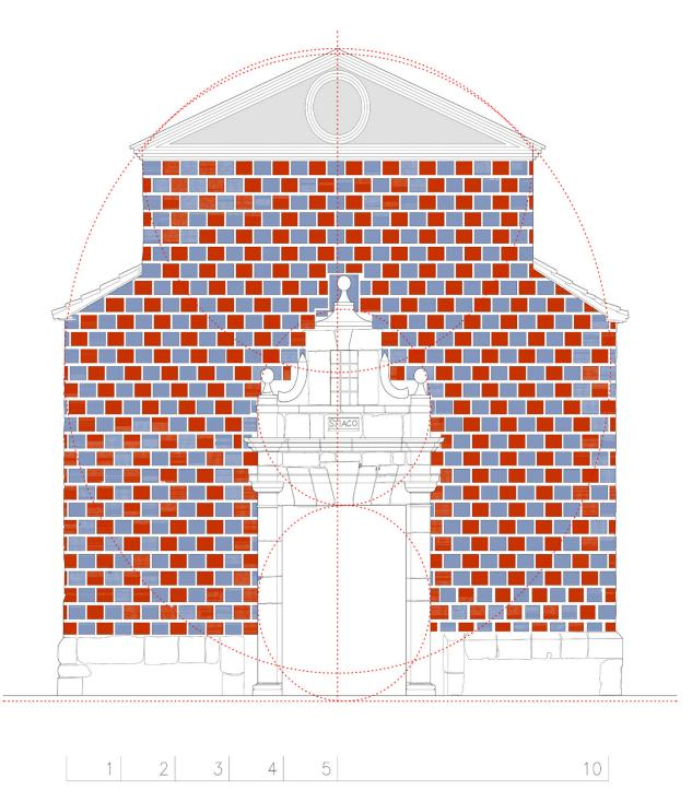
Fig. 11. A hypothesis of finishing the façade has been drawn by means of a pediment, adjusted to the general composition by means of a regulatory layout based on the circle - whose adjustment avoids the imperfections inherent to the physical reality of the building (Authors 2013).
