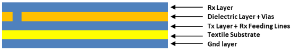
Figure 14. Cross-section of the 3DS-1 sensor. In addition to the 4 layers shown in Figure 13 the textile substrate between the ground plane layer and the Tx electrode layer can be observed.
