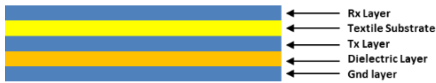
Figure 16. Cross-section of the 3DS-2 sensor. In addition to the 4 layers shown in Figure 15, the textile substrate between the Rx layer and the Tx electrode layer can be observed.
