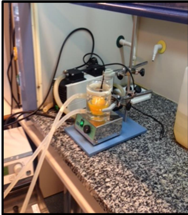
Figure 2.2: procedure of chemical bath deposition technique
