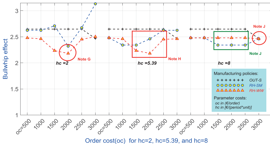
Figure 10. Bullwhip effect of manufacturing orders OUT-S, RH-SM, RH-WW in a scenario with ltv (2–4 weeks).
