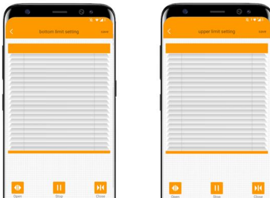
Figure 12. Detail of the upper and bottom limit setting in the BlindEngine App
