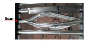
FIG. 25. Picture of the state of the T12-Ir3 target after a single beam impact of  $1.71 \times 10^{12}$  ppp.
