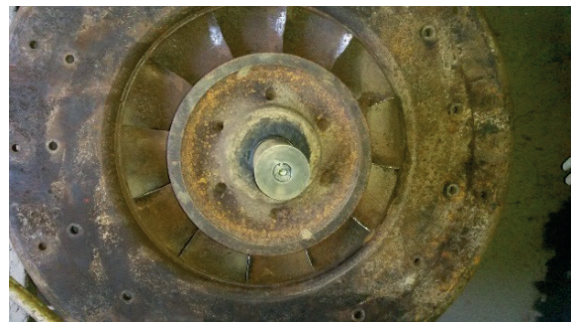
Figure 3: Francis turbine. (Source Endesa Generación-Enel Green Power).
