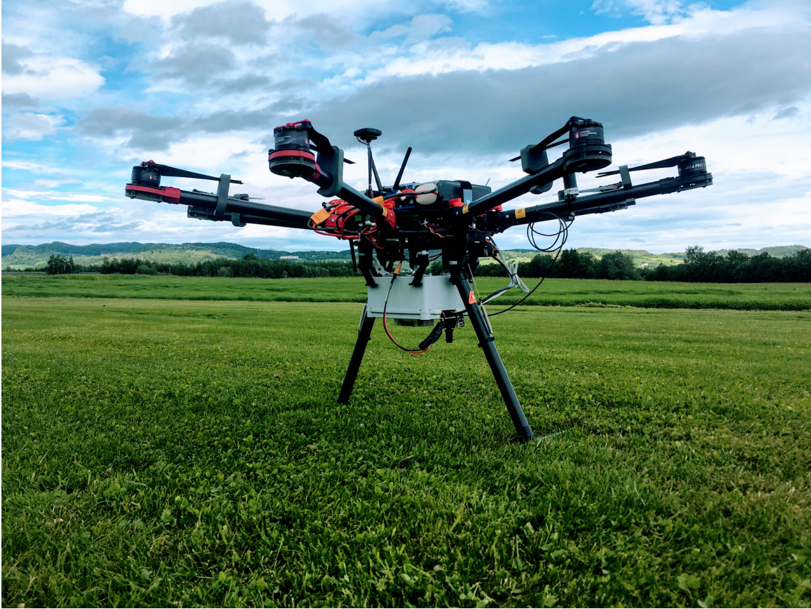
Figure 13: The S1000 with a hyperspectral payload. Credit: Elizabeth Prentice
