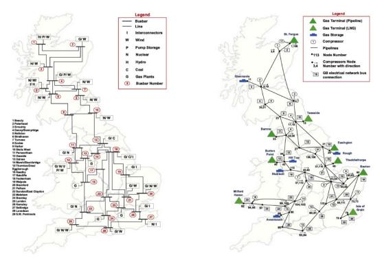
**Figure 4.** Geographical and functional infrastructure interdependence between the national electricity grid (**left**) and the gas transmission infrastructure (**right**) for Great Britain. Figure adapted from Reference [243].
