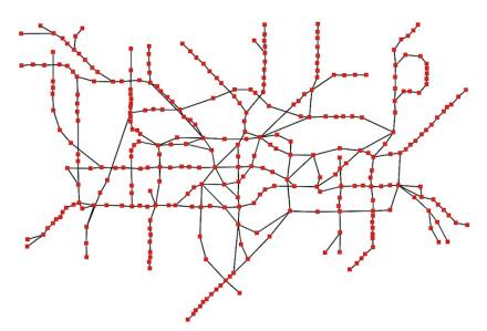
**Figure 3.** London underground scheme as example of complex network: The layout shows a quasi-planar (few crosses between links) as well as a core-periphery (more densely connected at the centre) structure.
