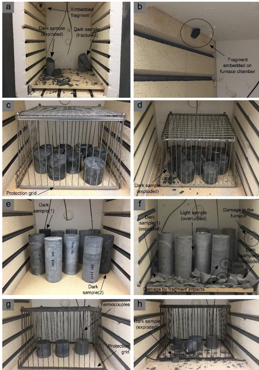
Figure 6. (a) Dark samples exploded or fractured when heated at 400° C. (b) Detail of the fragment embedded in the furnace chamber due to the violence of the event shown in (a). Dark samples before (c) and after (d) heating at 400°C. Note the protection grid used to preserve the furnace. Dark and light grey cores before (e) and after (f) heating at 500°
