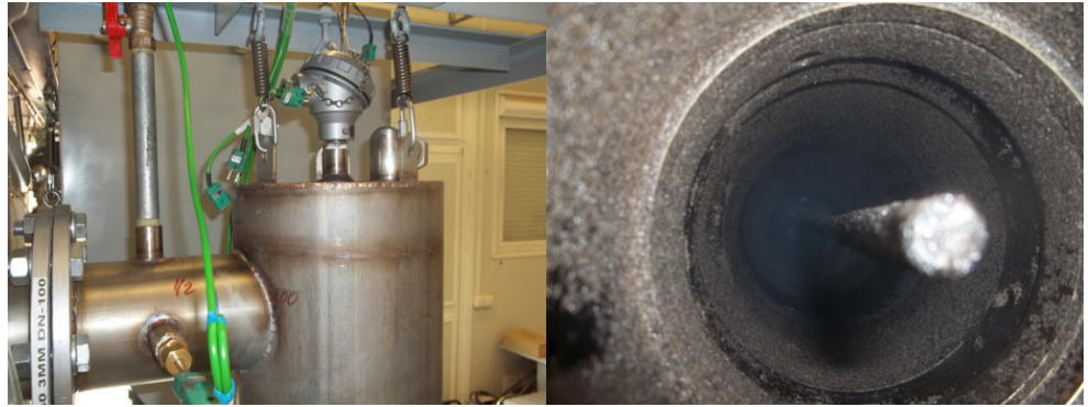
Figure 14. Thermocouples located in a thermowell: Top of the reactor ( Left ), inside the reactor ( Right ).
