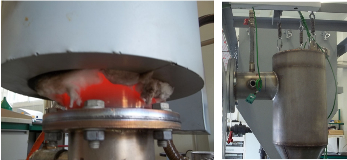
Figure 15. Bottom part of the reactor, when heated to red heat during the operation ( left ), Reactor holder system to absorb thermal expansion ( Right ).
