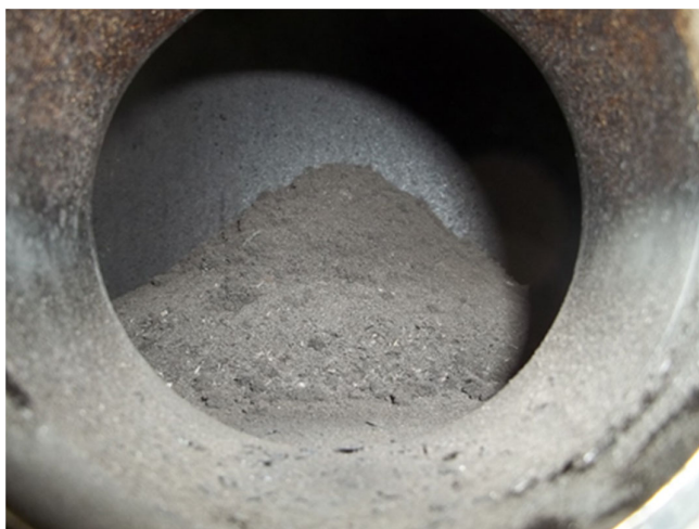
Figure 16. Cyclone discharge material.
