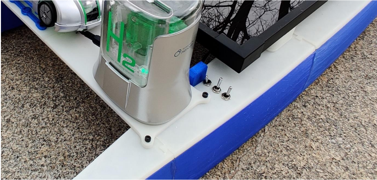
Figure 112: Mode pilot switches
