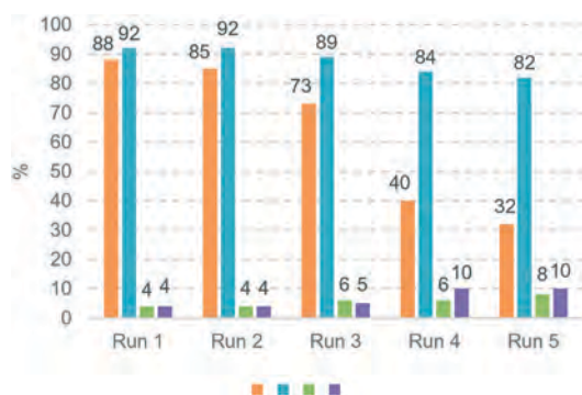
Fig. 6 Recycling experiments using Ni@L1 as the catalyst. Reaction conditions: 0.5 mmol of 3-hexyne, 3 mmol% catalyst, 0.75 mL toluene, 1 bar H 2 , and 5 h. Conversions and selectivities were determined by 1 H NMR (average of two runs).
