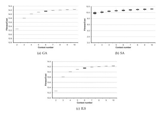
**Figure 4.** Fitness/cost dispersion vs. Context number applied to HL subband for neighborhood 5AR. (a) For GA algorithm. (b) For SA algorithm. (c) For ILS algorithm.
