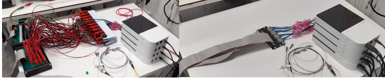
Figure 4.6: Luzwavelabs multicurrent connection before and after the connection integration.
