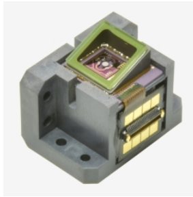
Figure 3.1: Example of Reconfigurable micro-mirrors [143].
